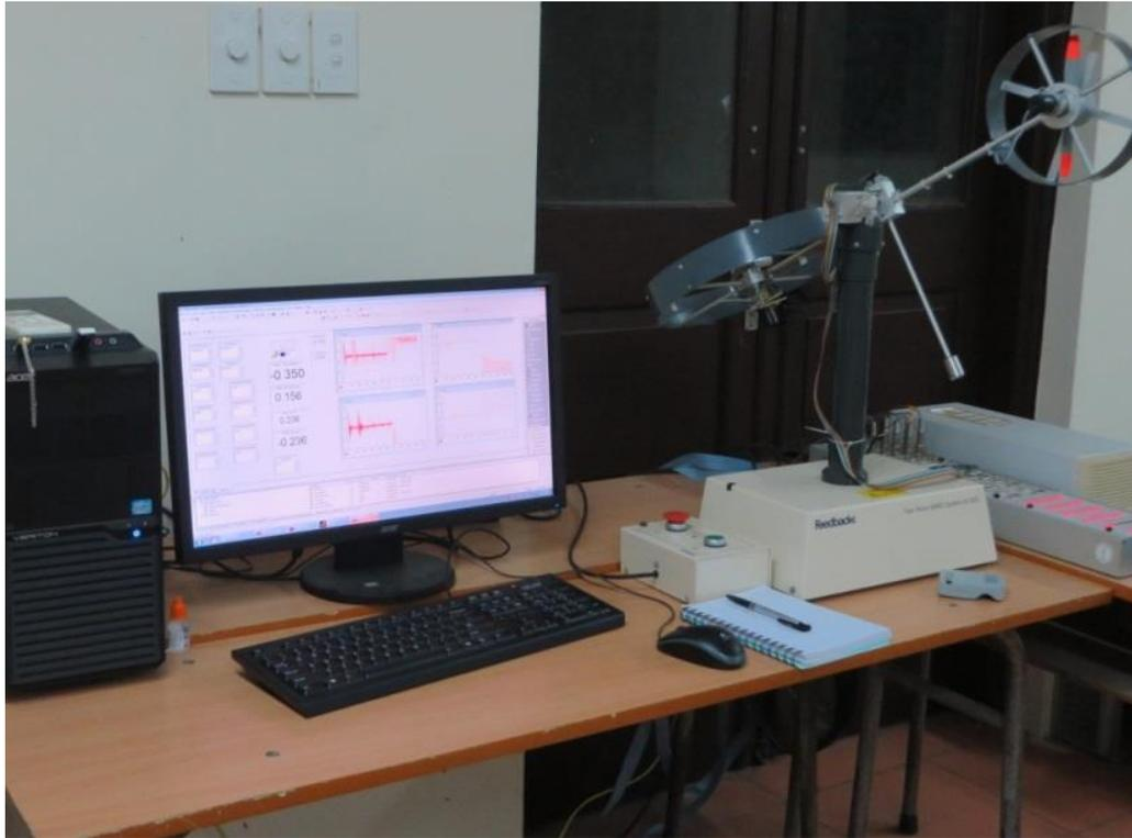
*Figure 4.13. The experimental system TRMS*
