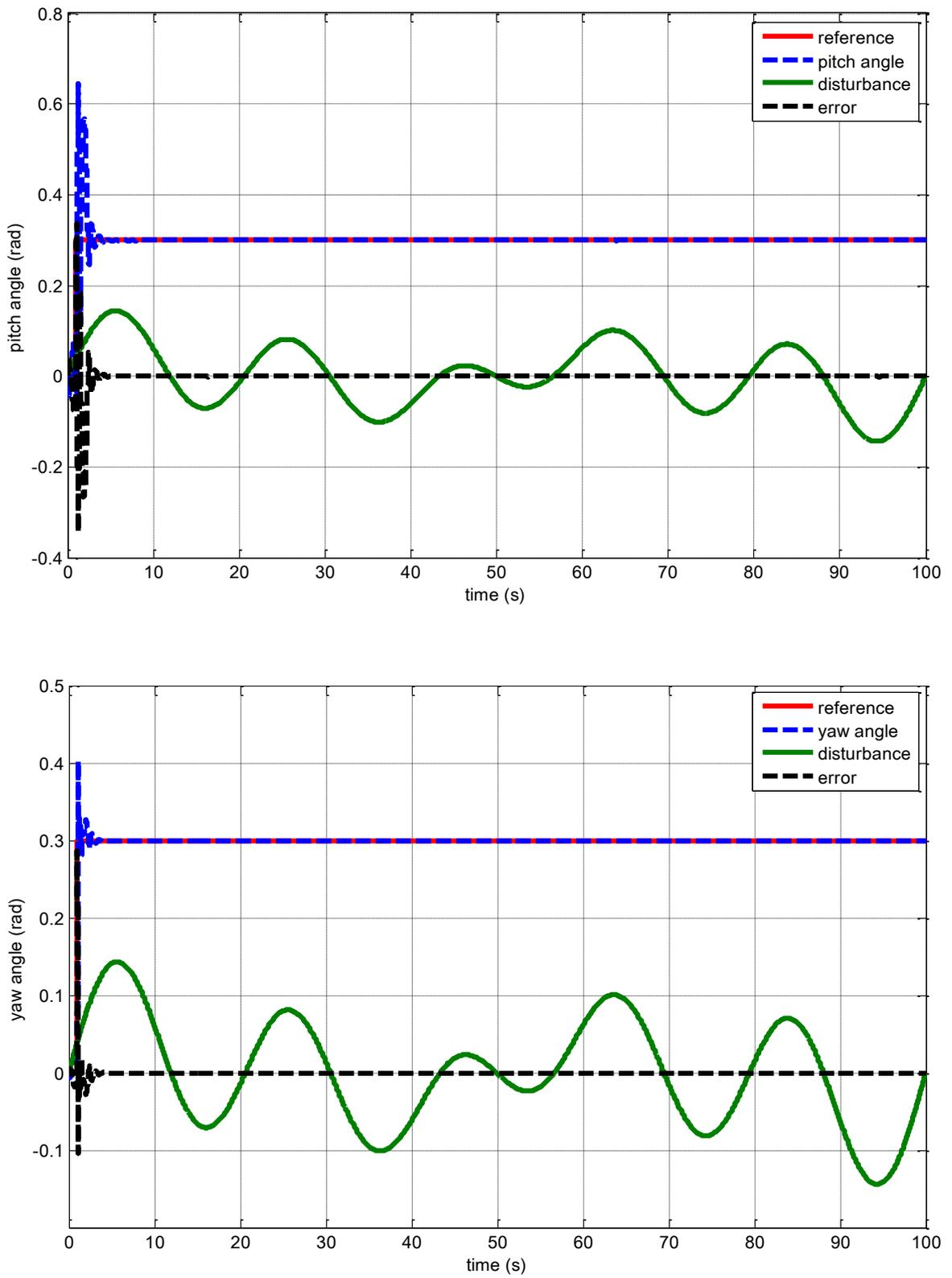
Figure 3.10. Output angle with step reference in 2 plane and disturbance
