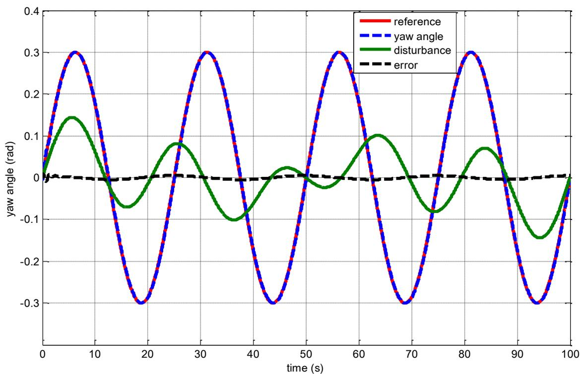
Figure 3.11. Output angle with sinusoidal reference in 2 plane and disturbance
