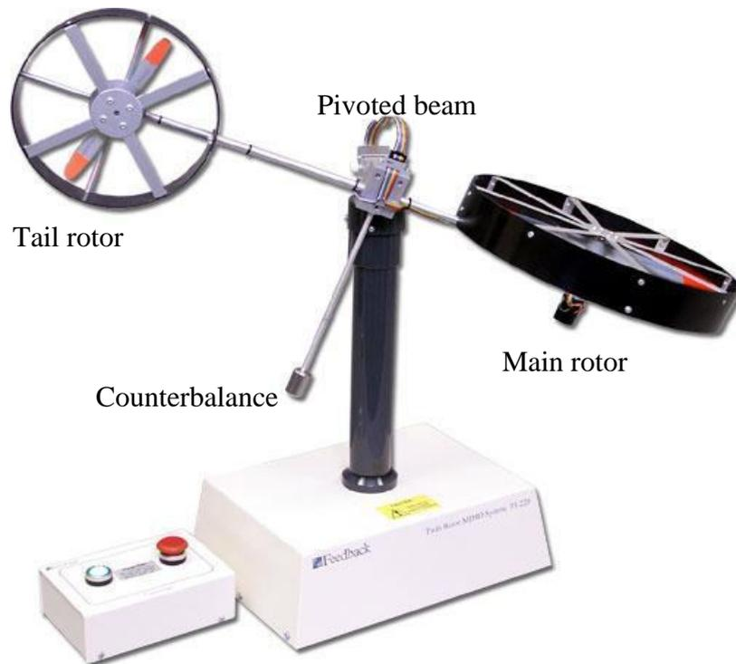
*Figure 1.1. Twin Rotor MIMO System (TRMS)*
