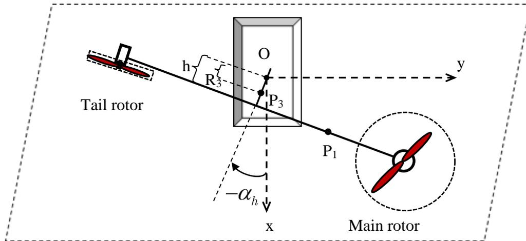
Figure 1.4. Angle position on horizontal plane  $\alpha_h$  of TRMS
