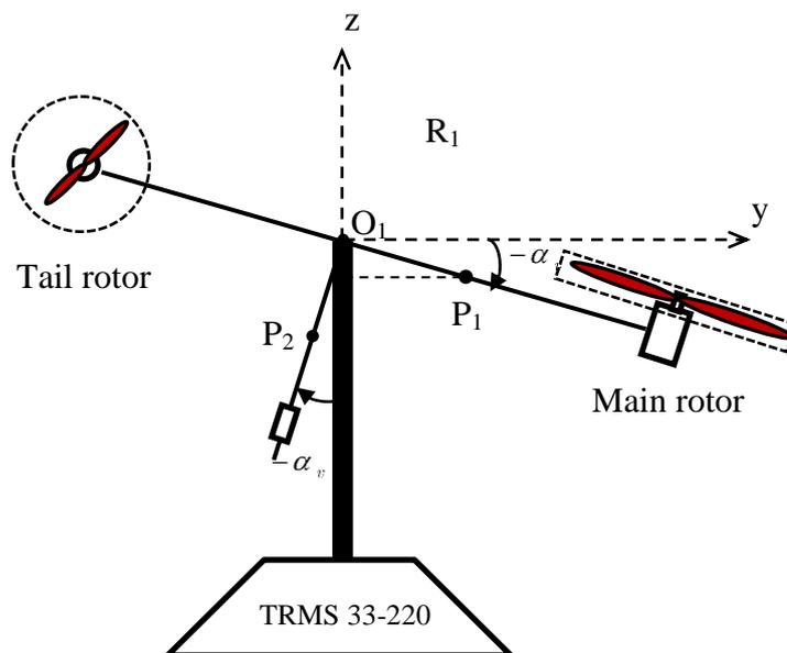
Figure 1.3. Angle position on the vertical plane  $\alpha_v$  of TRMS
