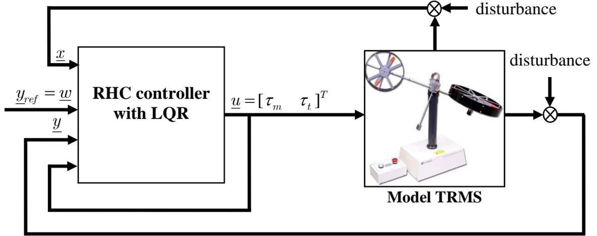
Figure 3.4. Control structure RHC with LQR for TRMS
