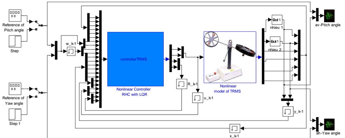
Figure 3.5. Simulation structure of control system TRMS with matrix  $R$  descending value
