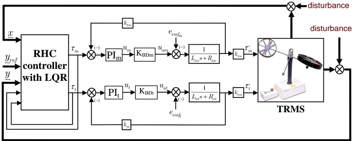
Figure 4.1. Control structure TRMS with an extra torque control loop
