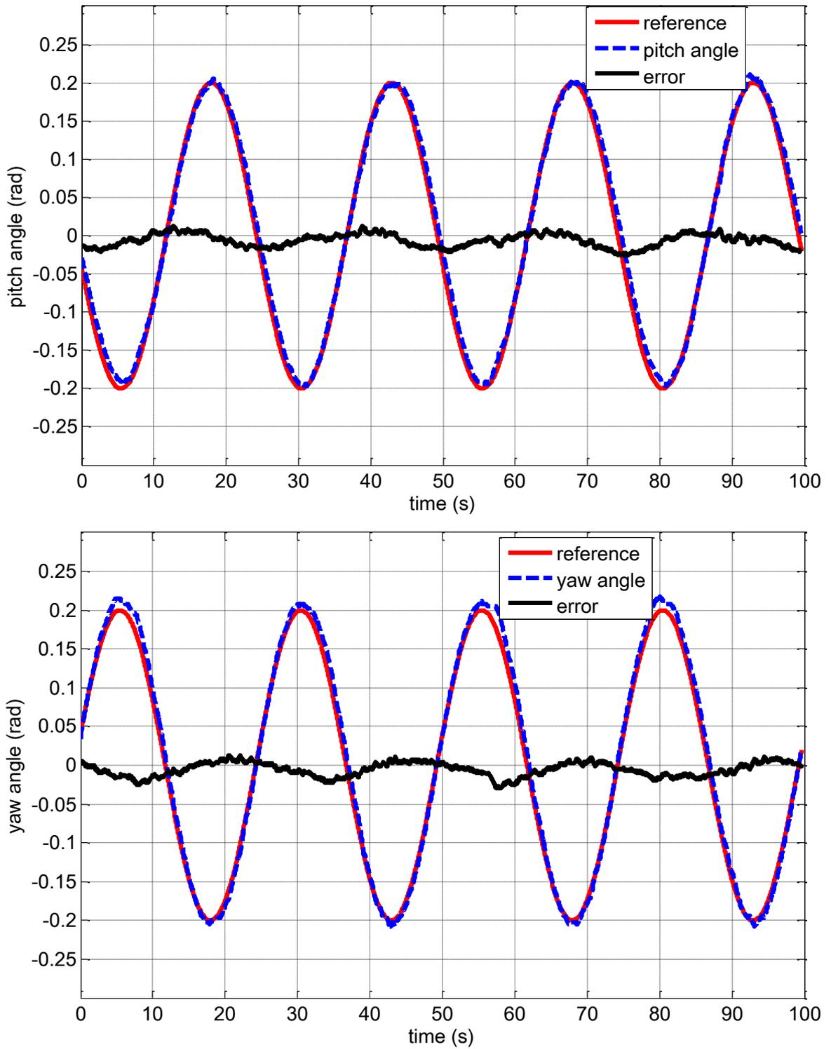
Figure 4.21. Response of angles in two planes with sinusoidal-sinusoidal signal references
